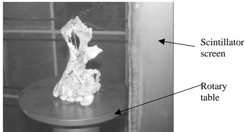
**FIGURE 1.** Fossil placed on rotary table.
